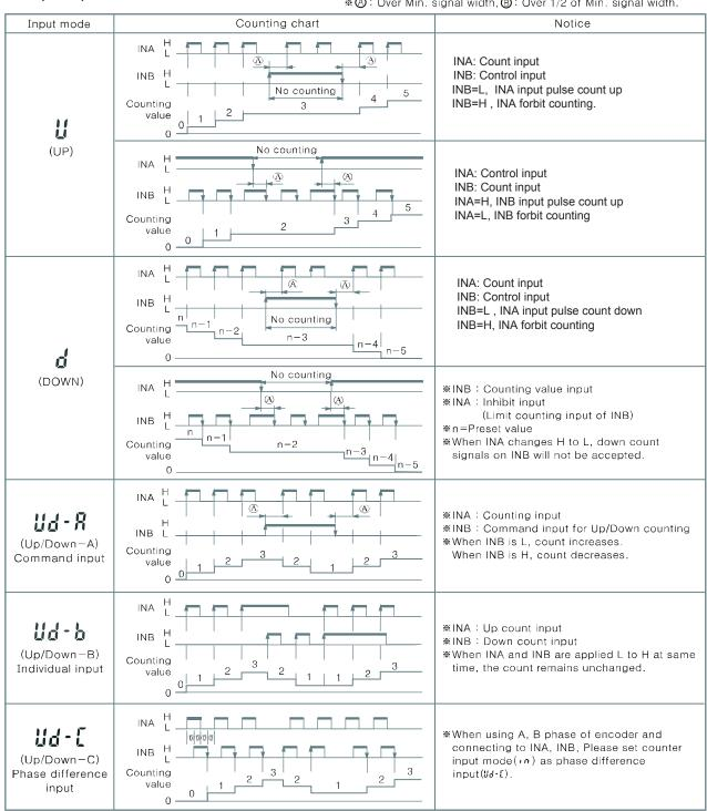
When you use an encoder and connect its phase A and Phase B output to the INA and INB input of the counter, please set the mode of the counter as Ud-C.
