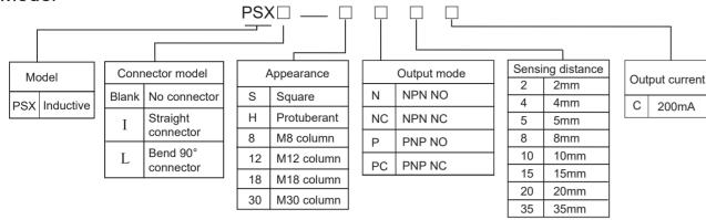
For example: PSXI-12N4C means inductive proximity sensor with straight connector, 12mm in diameter, NPN NO, sensing distance is 4mm, max output current is 200mA.
