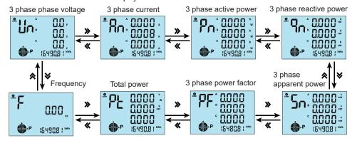
(note: in 3 phase 3 wire status only dislay 3 phase line voltage, current, total active power, reactive power, total power factor, frequency)
