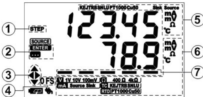
a) Digitals of last row: last time output signal , Digitals of bottom row: Currently setting&amending signal
