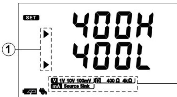
Above Row: High point parameter of necessary calibration
