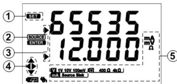
Above Row: high/low point DA code value of necessary calibration (0~65535)
