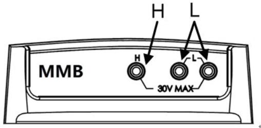
H: Output signal: Positive output terminal (+) ,
