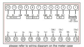
For voltage input terminals, the numbers in parentheses indicate 3 phase 3 wire connection method Mode 1 (3 pcs CT): 3 phase 4 wire connection mode 13 14 15 16 Current Input Voltage input 17 18 19 20 21 22 13 14 15 16 Current input via CT Voltage direct input Voltage input via PT Mode 2 (2 pcs CT): 3 phase 3 wire connection mode Current Input Voltage input 13 14 15 16 17 18 19 20 21 22 Current input via CT Voltage direct input Voltage input via PT
